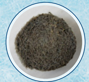
Cross-sectional area FIBALON® ball (used)
