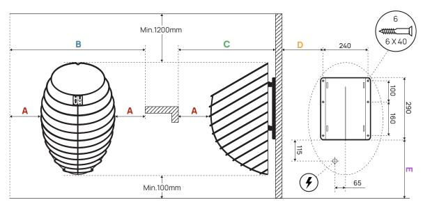
Figure 1. Positioning the heater
