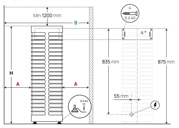
\* STEEL Mini 4 is attached to the wall with a special bracket See STEEL Mini 4 heater data in the table below.
