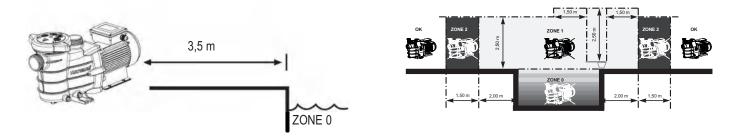
Install the pump in a ventilated and dry place. The motor requires air to flow freely around it to provide for natural ventilation. The pump has to be installed, so that the plug and the wall socket outlet is easily visible and accessible.
